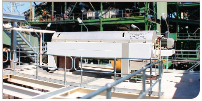
Faced with a tailings disposal problem, Rix's Creek believed that Alfa Laval's decanter centrifuges could help – and they couldn't be happier with the result.
